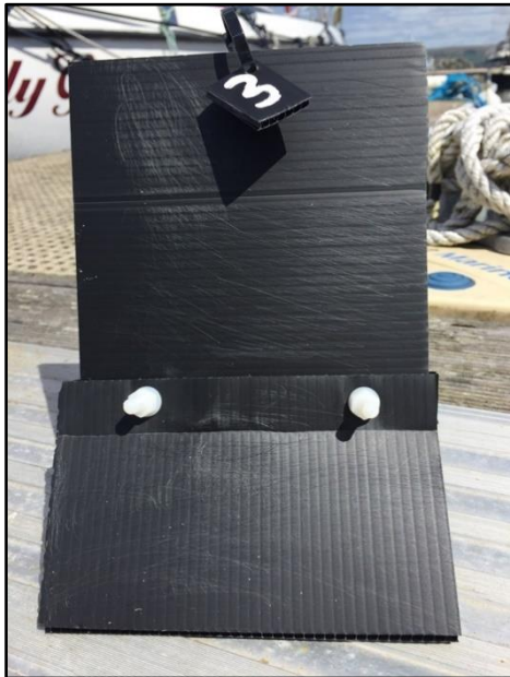
Photo 1 - Complex Correx panel structure
