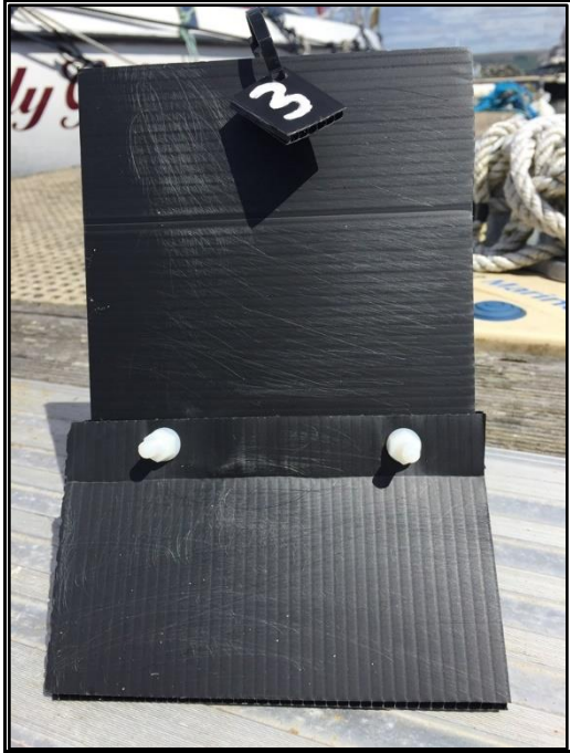
Photo 1– Complex Correx panel structure
