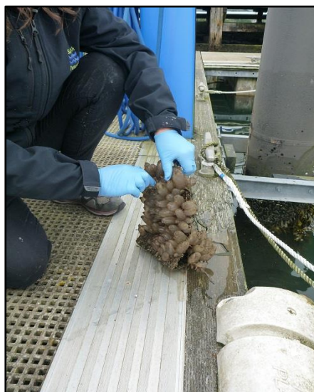
Figure 2: Checking a settlement panel in Stranraer Marina, Sept 2019
