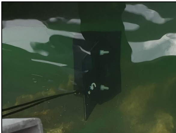
Photo 3 - Submerged complex Correx panel
