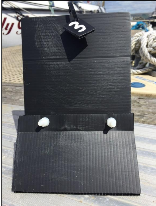
Photo 1- Complex Correx panel structure
