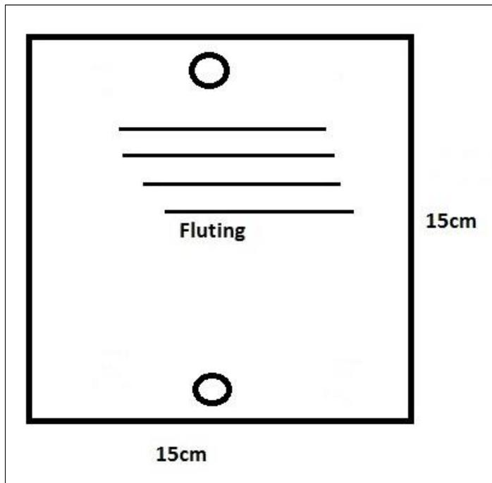
**Figure One – Correx panel structure (not to scale)**
